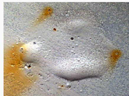
BLEED THROUGH AFTER AN IMPROPER REPAIR
