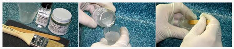
With both components, clear topcoat and hardener, at room temperature mix them at a 3:1 ratio and stir. Working time prior to hardening should be about 15 minutes.
