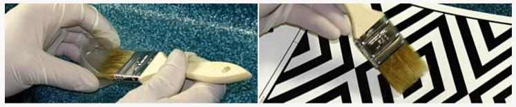
To perfect the topcoat application technique using the chip brush as a tool, perform a trial run on a separate surface for practice and repeat until an acceptable gloss and texture is achieved.
