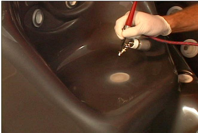
**Note:** Typically, two passes are required for full coverage. A dry film thickness of 0.002 "is generally adequate. Thinner coats will greatly increase the drying time.
