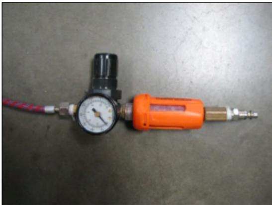
The airbrush should include a desiccant filter to avoid introducing moisture.
