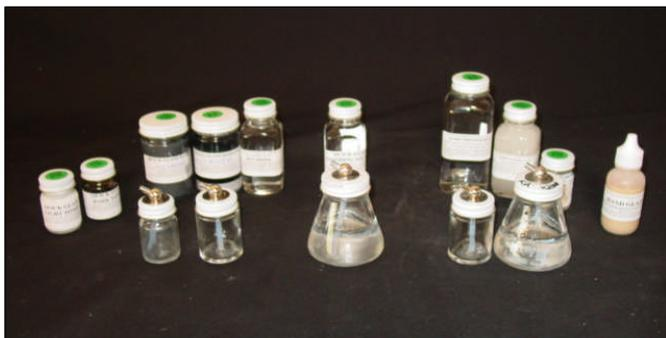
The materials needed to complete this repair include a primer coat, a base coat, and the K2000 topcoat. The **QUICK GLAZE** hardener is substituted with the K2000 hardener for the primer coat and base coats. The Quick Glaze Retarder is used to thin these color base coats in all temperature environments in replace of the **QUICK GLAZE** Reducers. The **QUICK GLAZE** Finishing Solvent is required to allow “feathering” to minimize the paint “halo”
