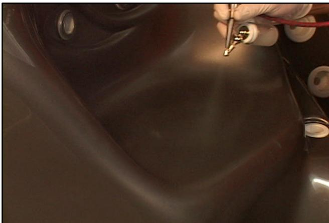
Feather the clear topcoat to create a smooth transition around the outside edge into the final gloss finish. Immediately spray the Thinner / Reducer for the Finishing Solvent liberally to achieve a smooth gloss and remove overspray. Be sure to wet the dry areas to match the original finishing gloss.
